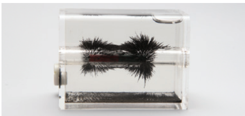
Experiment to illustrate magnetic field lines
