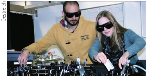
Ultrafast spectroscopy on GaN quantum wells for blue LEDs
