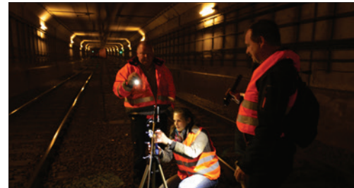
Meteorological measurements in a subway station
