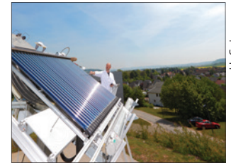
Testing a solar thermal vacuum collector
