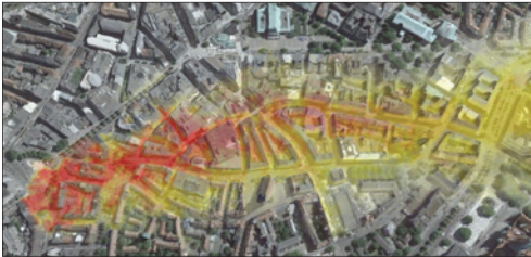
Pollutant concentration (red: high values) at street level in Hannover's old town district. PALM simulation of a virtual hazardous accident at Steintor place.
