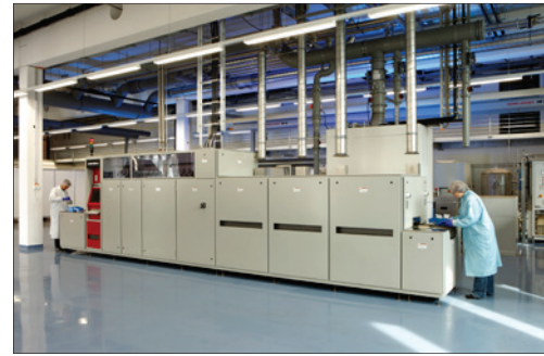
Firing oven in our research line for fabricating Si solar cells.
